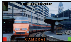
The IMD, 8-channel audio level meter, and time code display.*
