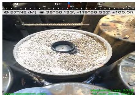
Loose clean media
