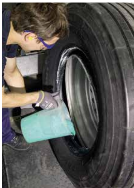
Inserting Ultra-Seal sealant into a super single trailer tyre
