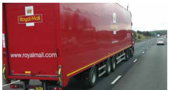
DAF CF85.410 with Cartwright's 15.65m Longer Semi-Trailer (LST) for the Royal Mail
