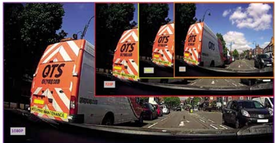
The above image illustrates the different resolutions at which the new DVRs can record (current generation DVRs record at D1 resolution)
