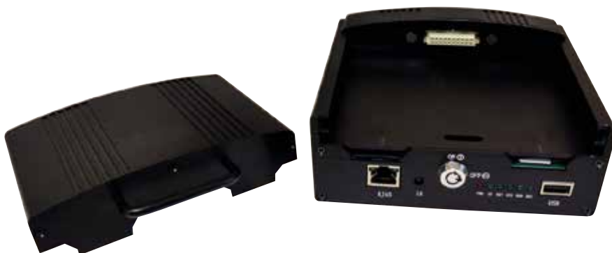
New DVR housing and cassette, with improved access to SIM card and SD card
