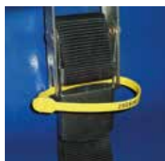
Integer polypropylene ring seal on curtainsider
