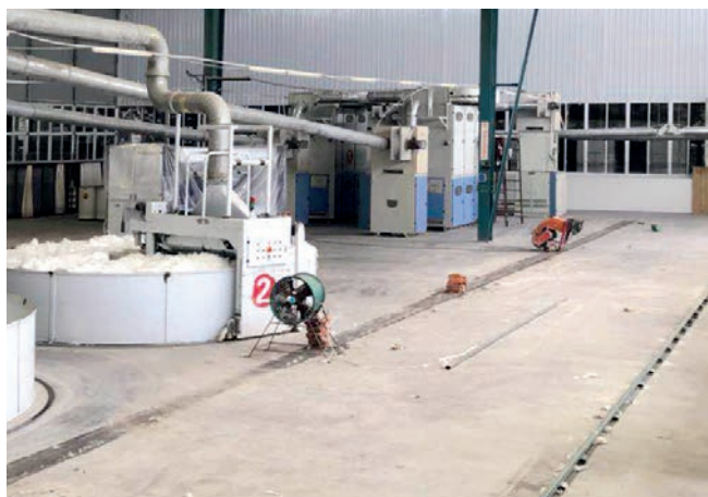
BO-P is installed at Hunan Huayi and must be modified in the blowroom line; the path is next to the wall
