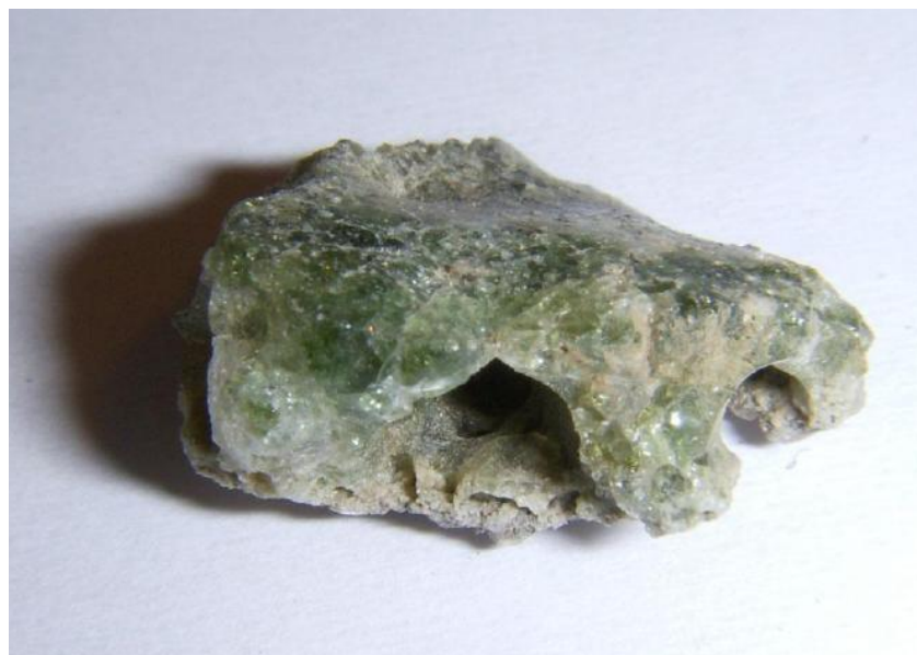
Figure 10c : A sample of trinitite glass from the trinity test site in New Mexico
