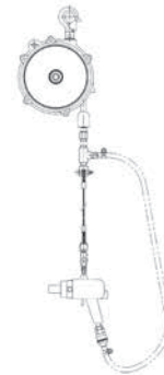
ATB-1 fitted with horizontal tool hanger
