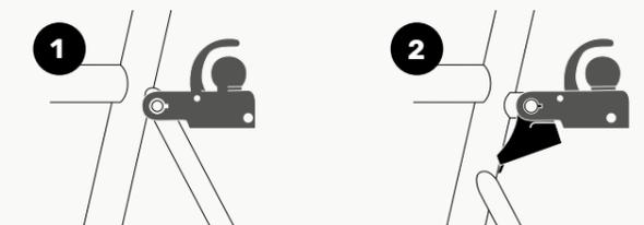
*To guarantee the coupling's whole angle mobility mount the coupling corresponding to the pictures undermentioned. Does the coupling not lay in the way like shown in **picture 1** you have to mount the support stand. In horizontal level the under part of the coupling has to lay on the seat stays (**picture 2**, support stand).*
