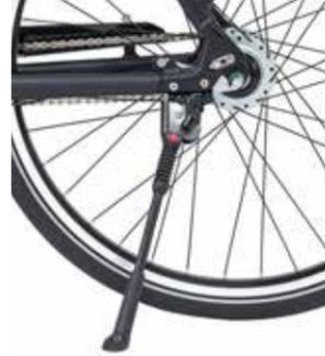
*Form-fit stand solution for direct dropout fixing KSA 40 (= special adapter on the chain stay, hole spacing 40 mm), incl. 2 x screws M6 x 16.*
