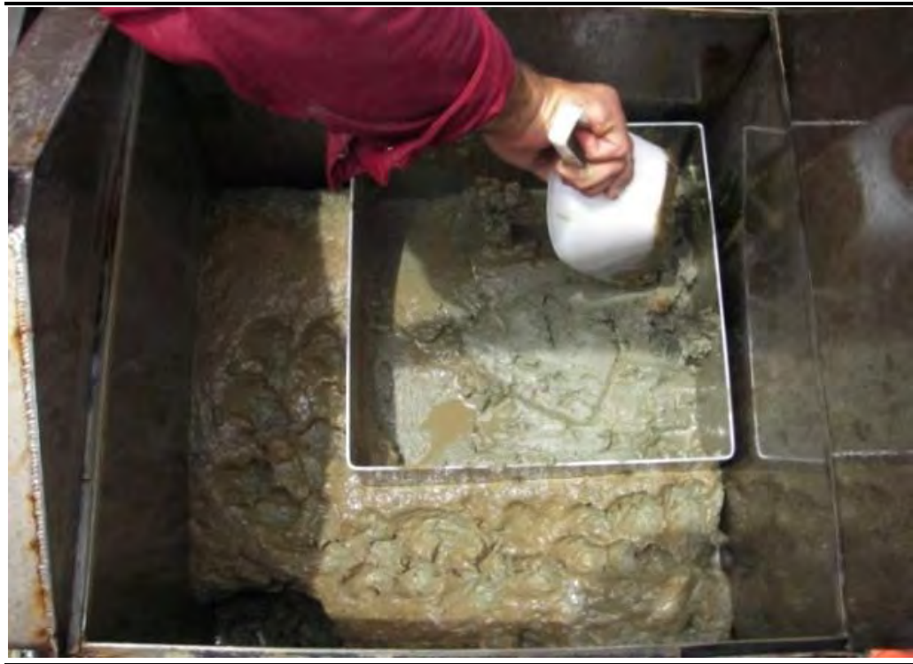
Figure 4.23 Collection of Macroinfaunal Samples from an Insert within the Box Core Sample
