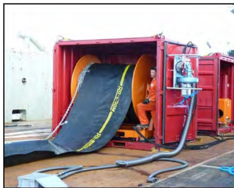
Ro- Boom 1500 deployed offshore
