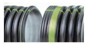
Provides excellent flow and durability for rapid outlet and transfer of collected water. Available with standard plain end or soil-tight built-in gasketed bell and spigot joints for quick installation. Delivered in 20' lengths, 4" through 60" diameters, perforated or non-perforated.
