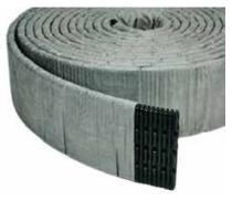
A perforated panel-shaped polyethylene core in 12" and 18" widths and in coils up to 100'. Can be used with or without a covering geotextile sock for filtration of fines. 12" AdvanEDGE has twice the response rate of 4" round pipe, removing a given quantity of water 60% faster. AdvanEDGE can be installed vertically in narrow trenches for field and perimeter drainage, or laid flat directly on the subgrade of greens and bunkers.
