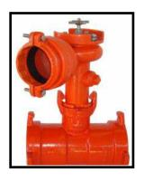
Lateral Valve spigot inlet inserts into the lateral tee or lateral saddle outlet. If the valve remains in the original installed position, two LV-Clips are needed to secure the valve in place. LV-Clips slide between the lugs of the lateral outlet to prevent the valve from dislodging. LV-Clips are sold separately.
