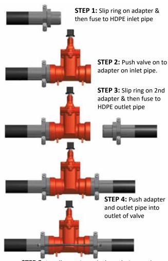
**STEP 5:** Install restraint rods through rings and tighten once to 40 ft-lbs.
