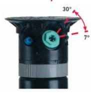
From 7° to 30° in 1° increments put water where you want it. Adjust from the top of the sprinkler in seconds - wet or dry. This flexibility lets you tackle every obstacle on the course; wind, trees, bunkers, mounds and more.
