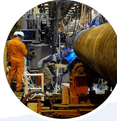
Onboard *Pioneering Spirit*, the pipe joints are welded together.
