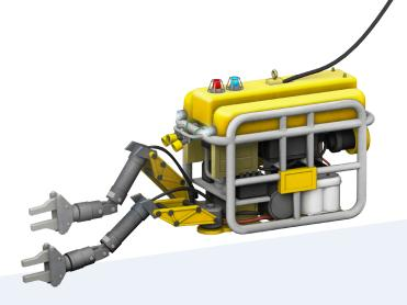
Using a remotely operated vehicle (ROV) is one of the methods we use to investigate the seabed in detail. The ROV makes it possible to film in the deep seas. It can also carry other instruments such as sonar and a magnometer. We make sure that all relevant objects are identified.
