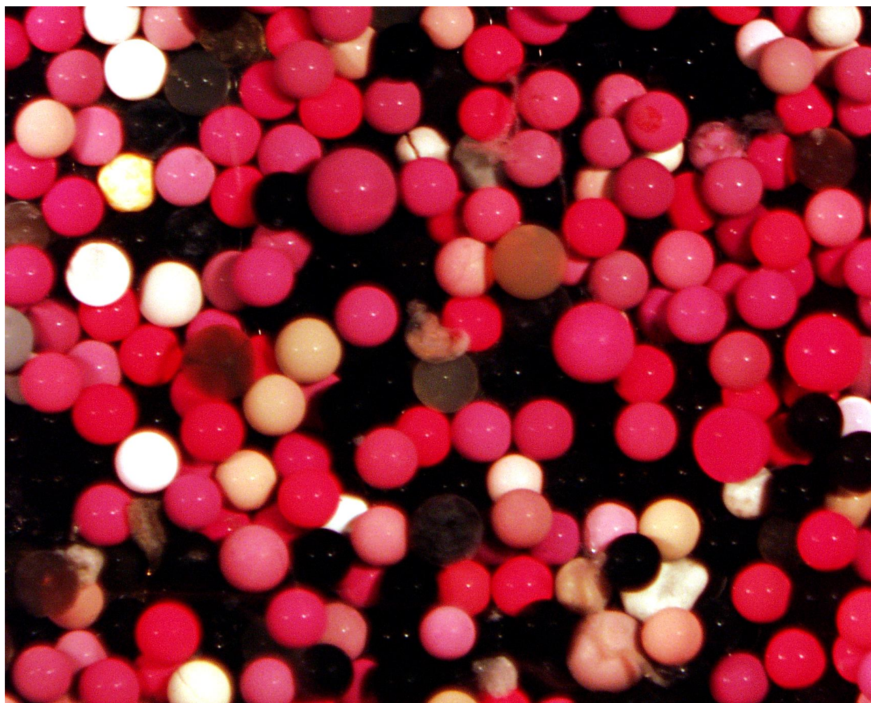
Figure 38. Plastic spheres found at the Formosa Discharge station FD in the HRI study. Spheres are about 0.5 mm in diameter.
