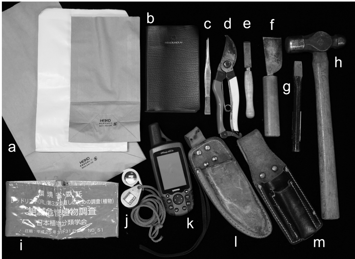
Fig. 3. Collection tools. a: paper bags; b: field notebook; c: tweezers; d: secateurs; e:
