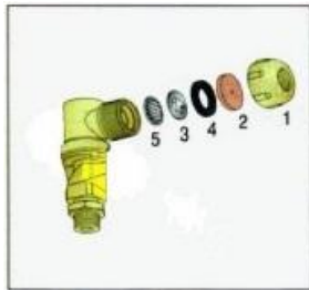
Fig.4 Construction of the LC nozzle:
