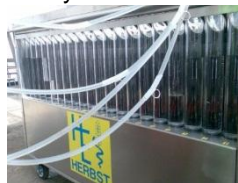
Fig.3 Ramp with the liquid collector cylinders
