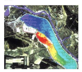
Lake: This image shows the thermal discharge from a nuclear plant into a lake. The warm water (red) discharged from the circulating water system enters the lake via a long canal and then cools as it flows counterclockwise around the lake, guided by a long weir wall. The cooled water (dark blue) is drawn back into the plant's intake structure for another cycle.
