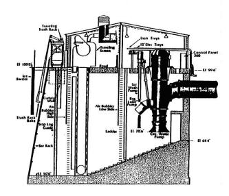
buildup on the traveling screens. Nuclear power plants use two to four circulating water pumps for each reactor unit. Each circulating water pump with its electric motor stands nearly 40 feet tall and supplies over 100,000 gallons of water. The piping from the discharge of the circulating pumps runs underground from the intake structure to the turbine building.
