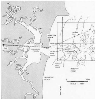
Ocean: This drawing shows the underground piping routed from offshore intake and discharge points for a coastal nuclear plant. The intake and discharge points in this case are nearly one mile offshore.
