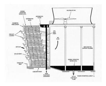
PART SECTION OF A NATURAL DRAUGHT COOLING TOWER - COUNTER FLOW
