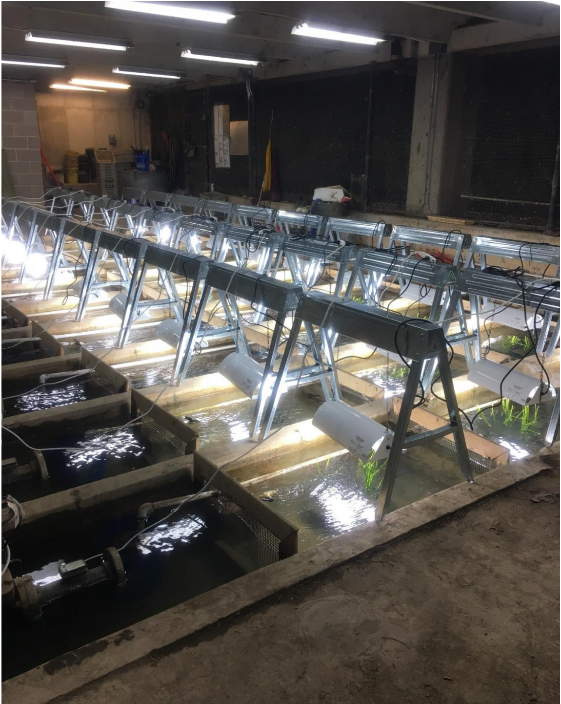
Figure 6. Photo of stream channel set up at raceways at Texas State University in San Marcos. The head of each stream channel has a sump pump that leads into PVC pipe and then out a ball valve in each cell. The dividers are set up to divide each channel into three different cells of equal dimensions. The lights are hung 30 cm over each stream channel to ensure equal light for each cell.
