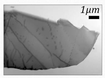
Once thinned to ~100-150nm, the section was analyzed using transmission electron microscopy. Bright field STEM images of section 1 are shown (above and to the right)
