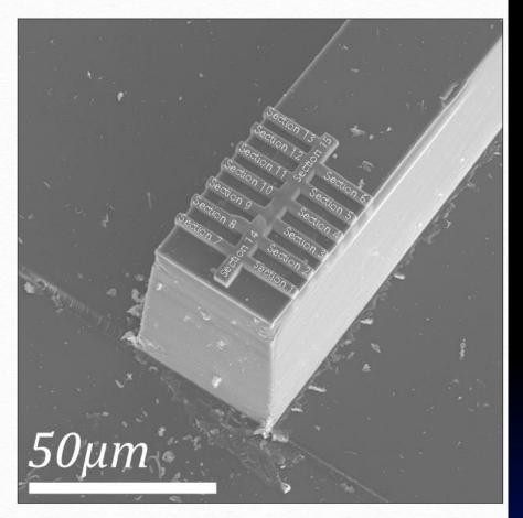
A protective carbon cap has been placed over the areas of interest. The locations of the 15 planned FIBprepared electron transparent thin sections are indicated
