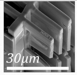
Material between sections 1 through 6 was been milled away (left). Then material under section 1 was milled away in preparation for lift out (above).
