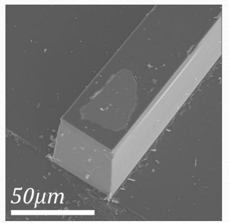
Oblique view of the grain after being embedded in epoxy and partially sectioned. The material surrounding the grain has been removed, leaving it at the end of a rectangular box sitting on top of the bulk of the substrate.
