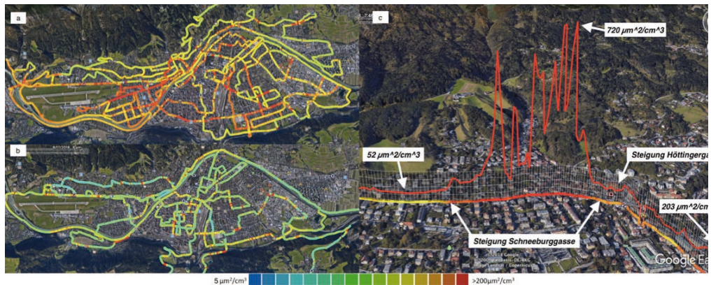
Figure 2: LDSA-Concentration during different Conditions. (a) shows the morning distribution of a summer day. (b) illustrates the nanoparticle “hot-spots” of a summer day afternoon. (c) is an example of vehicle plumes caused maxima on an uphill street
