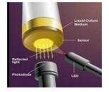
The bottles have pH-sensitive membranes in the bottom of the bottles. Microbial growth causes a release of  $CO_2$ , which changes the pH in the sensor and color from gray to yellow. The color change is measured by reflected light. The level of  $CO_2$  is measured colorimetrically.
