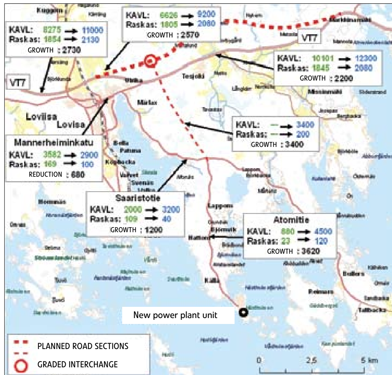
Figure 8-4. Average weekday traffic (KALV) and the volume of heavy traffic (Raskas) in 2006 and in the fourth construction year of the new power plant unit.
