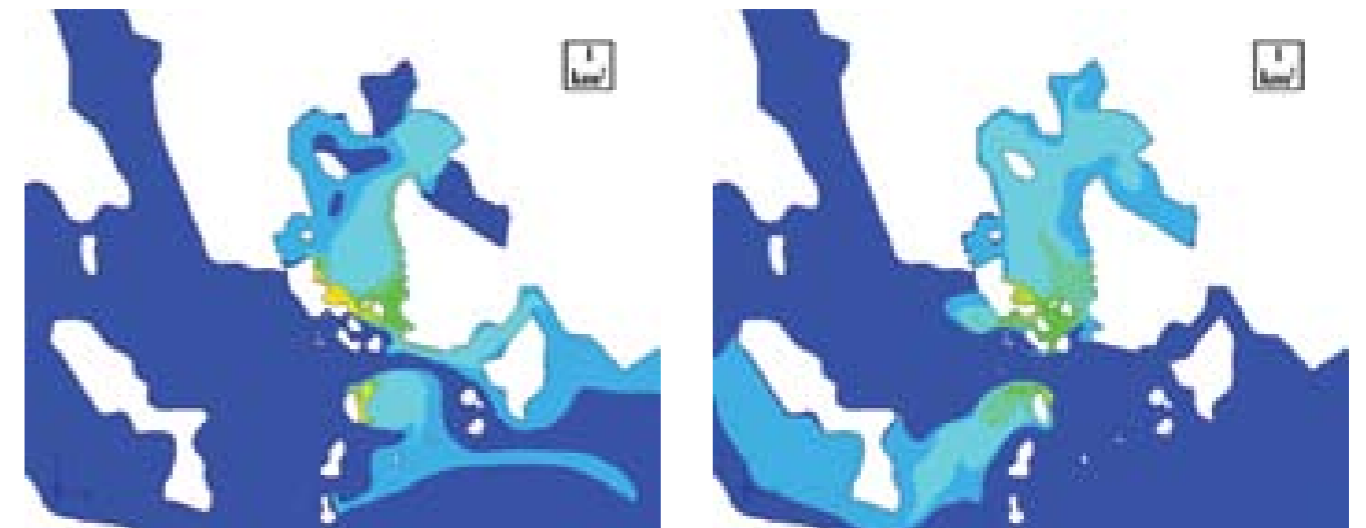
Figure 9-6. Summer (LR). The impact of the existing power plant units and Loviisa 3 (O1, P2) on sea water temperature during a southeast wind (left-hand picture) and northeast wind (right-hand picture).
