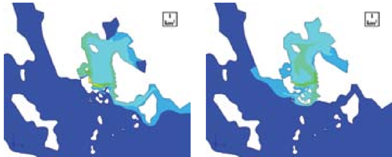
Figure 9-7. Summer (RL). The impact of the existing power plant units and Loviisa 3 (O2, P1) power plant unit on the temperature of sea water during a southwest wind (left-hand figure) and northeast wind (right-hand figure).
