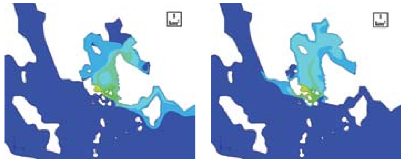
Figure 9-8. Summer (RR). Impact of the existing power plant units and Loviisa 3 (O2, P2) on sea water temperature during a southwest wind (left-hand figure) and northeast wind (right-hand figure).
