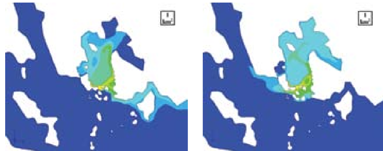
Figure 9-4. Summer, present situation. The impacts of the existing power plant units on the sea water temperature with a wind from the southwest (left-hand figure) and from the northeast (right-hand figure).
