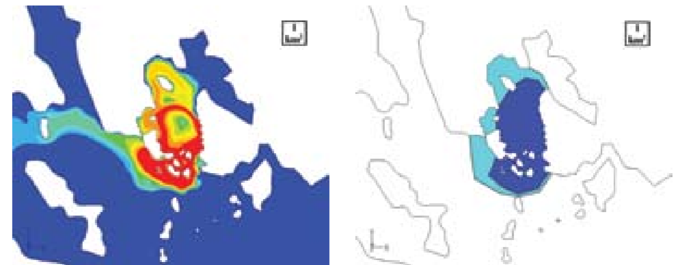
Figure 9-9. Winter, present situation. The relative temperature distribution caused by the existing power plant units (left-hand figure) and ice cover in the surroundings of Hästholmen (right-hand figure) based on observations during winters. In the figure describing the ice cover, the dark blue color represents open water and light blue open water or weak ice.
