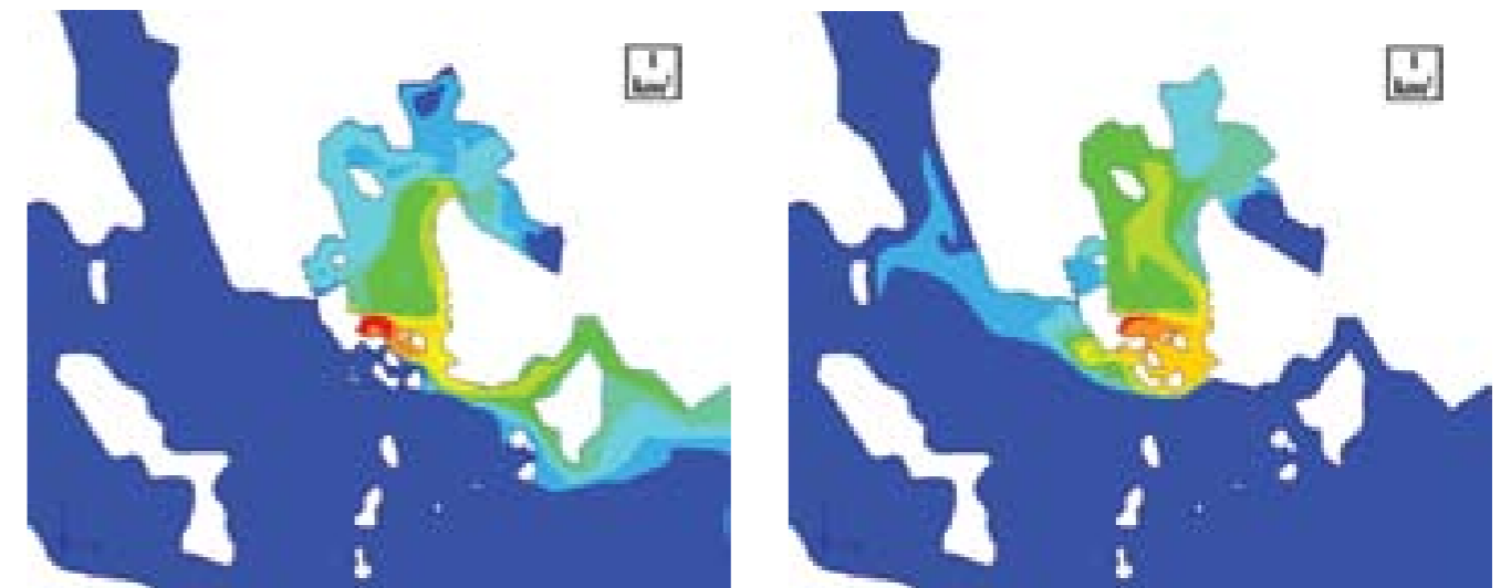
Figure 9-5. Summer (LL). The impact of the existing power plant units and Loviisa 3 (O1, P1) power plant unit on the sea water temperature during a southwest wind (left-hand figure) and northeast wind (right-hand figure).
