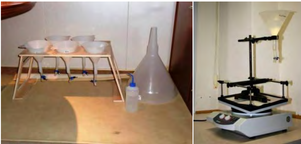
Fig. 21: Left: Travel-Baermann equipment used for collecting suspended soil organisms in efficiency-test samples. Right: Equipment used during the preliminary tests.
