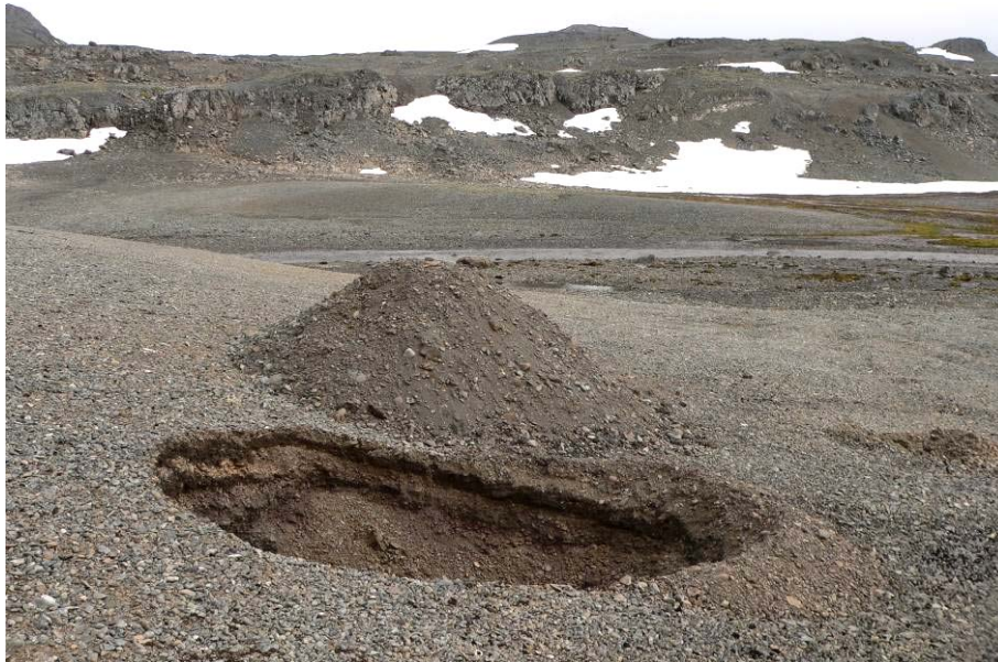
Fig. 4.4.-16: Test pit for construction material in the beach ridge complex, eastern Südpassage (photo: Buesser)
