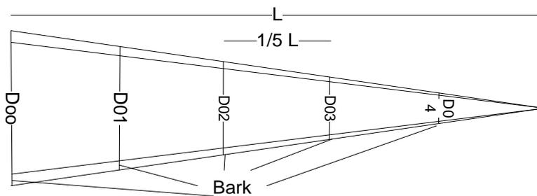
**Figure 4: Division method of felled stem into 5 equal lengths for calculating volume**
