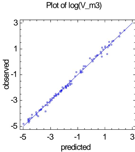
Figure 14: Linear regression between observed V with predicted V of equation  $V = f(\text{DBH}, H)$
