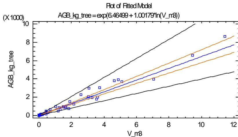
Figure 203: Fitted model between observed AGB and V
