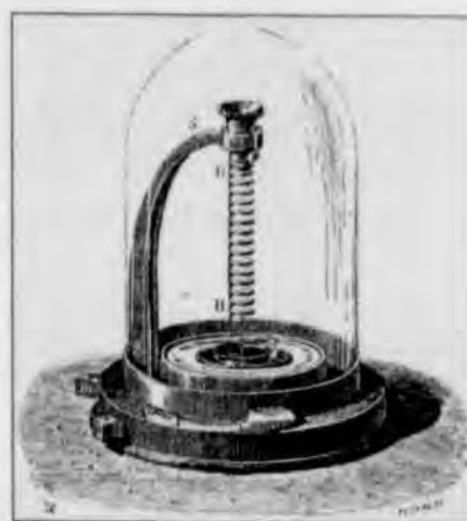
Fig.2 Breguet's metallic thermometer (From: Catalogue Breguet (Paris, 1877), p. 49).
