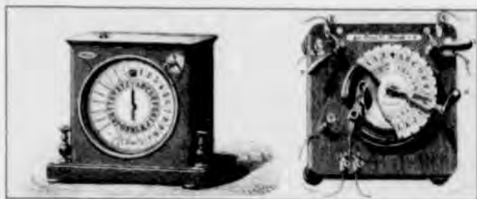
Fig.3 Breguet's dial telegraph (From: Interdisciplinary Science Reviews , op.cit., note 1, p. 158).
