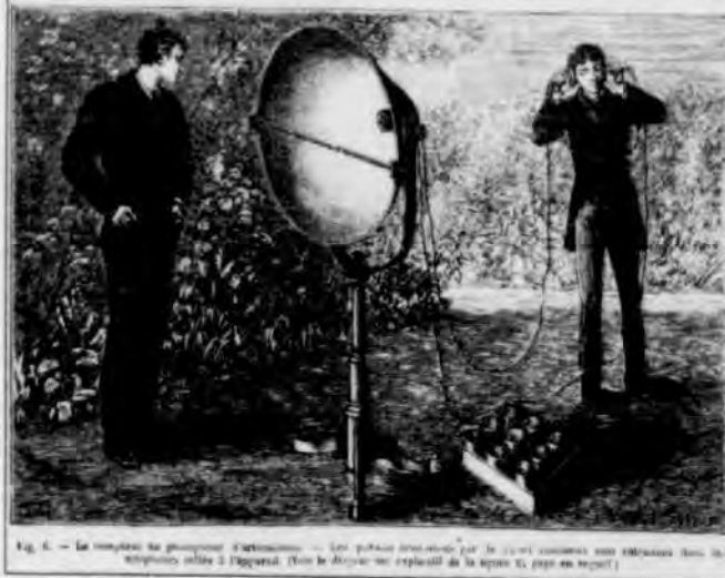
Fig.7 Bell's photophone made by Breguet. (From: La Nature, op. cit., note 28, page 345).
