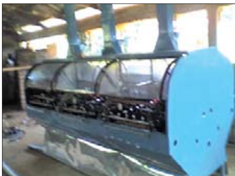
Re-reeling unit installed at the Kakamega Marketplace
