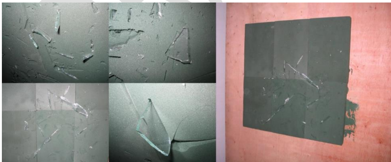
Figure 1: Glass shards penetration of surfaces after an explosion.
