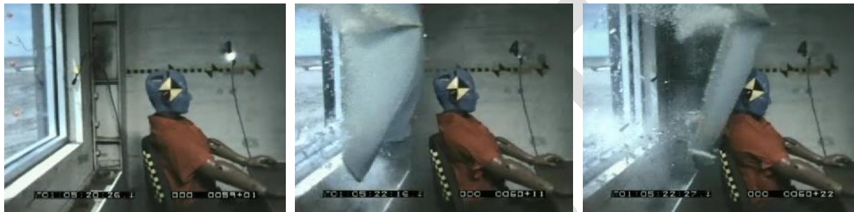
Figure 13: Examples of rigid catcher system, anchored horizontally.
