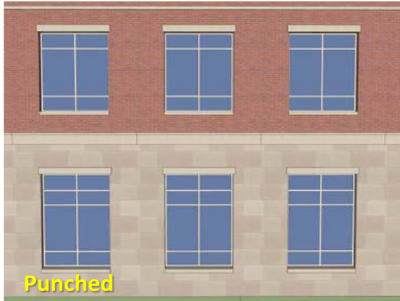
Figure 2: Types of window glazing
