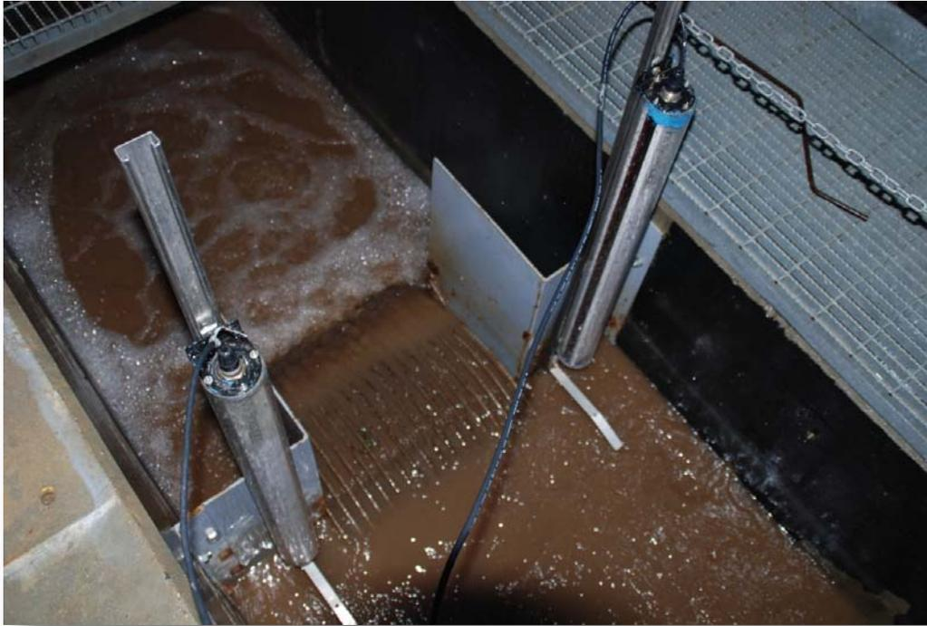
Photo 7 - Upstream Migration Monitoring Infrared Scanners
