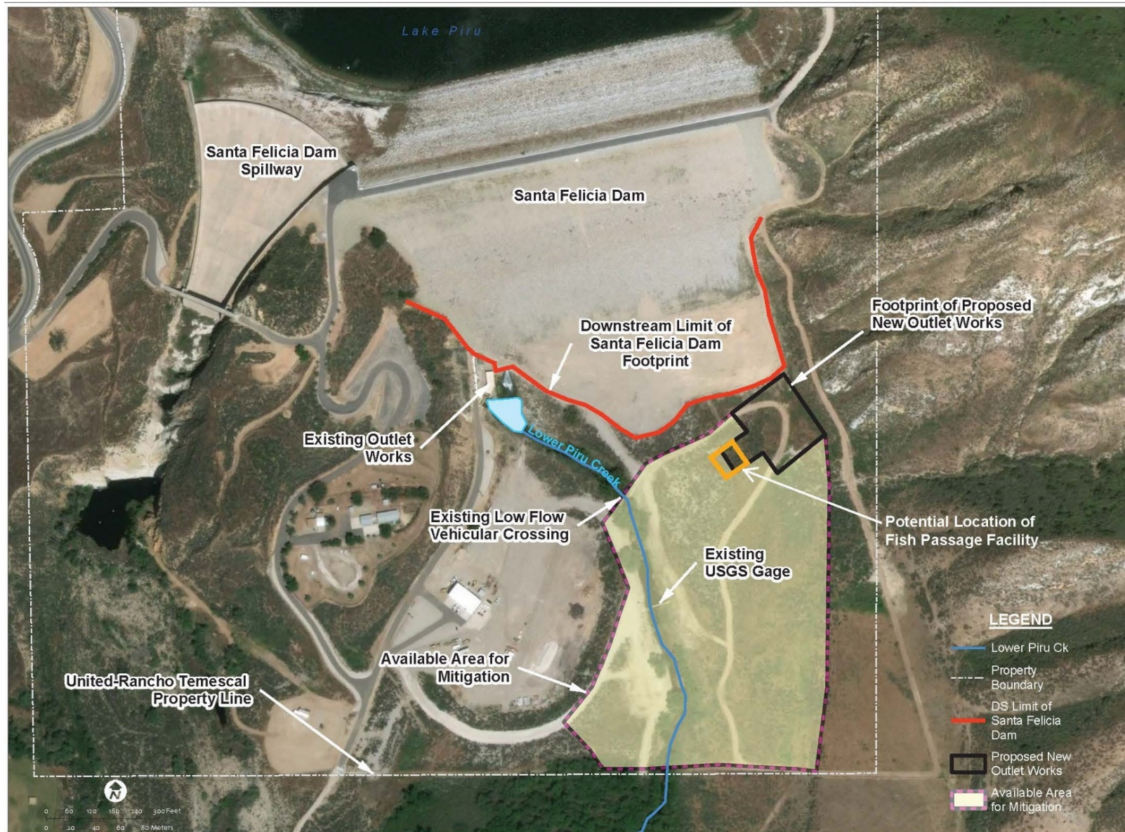
Figure 5.5-3 Location of New Outlet Works and Available Area for New Release Channel
