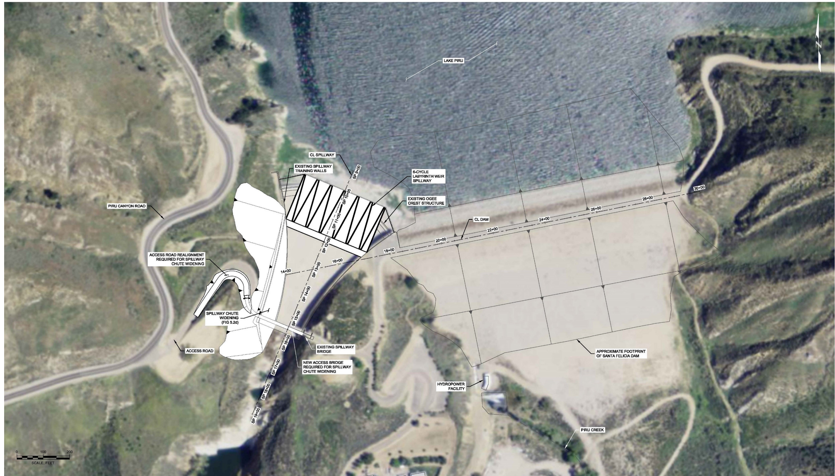
Figure 4-1 Labyrinth Weir Spillway and Spillway Widening Option
