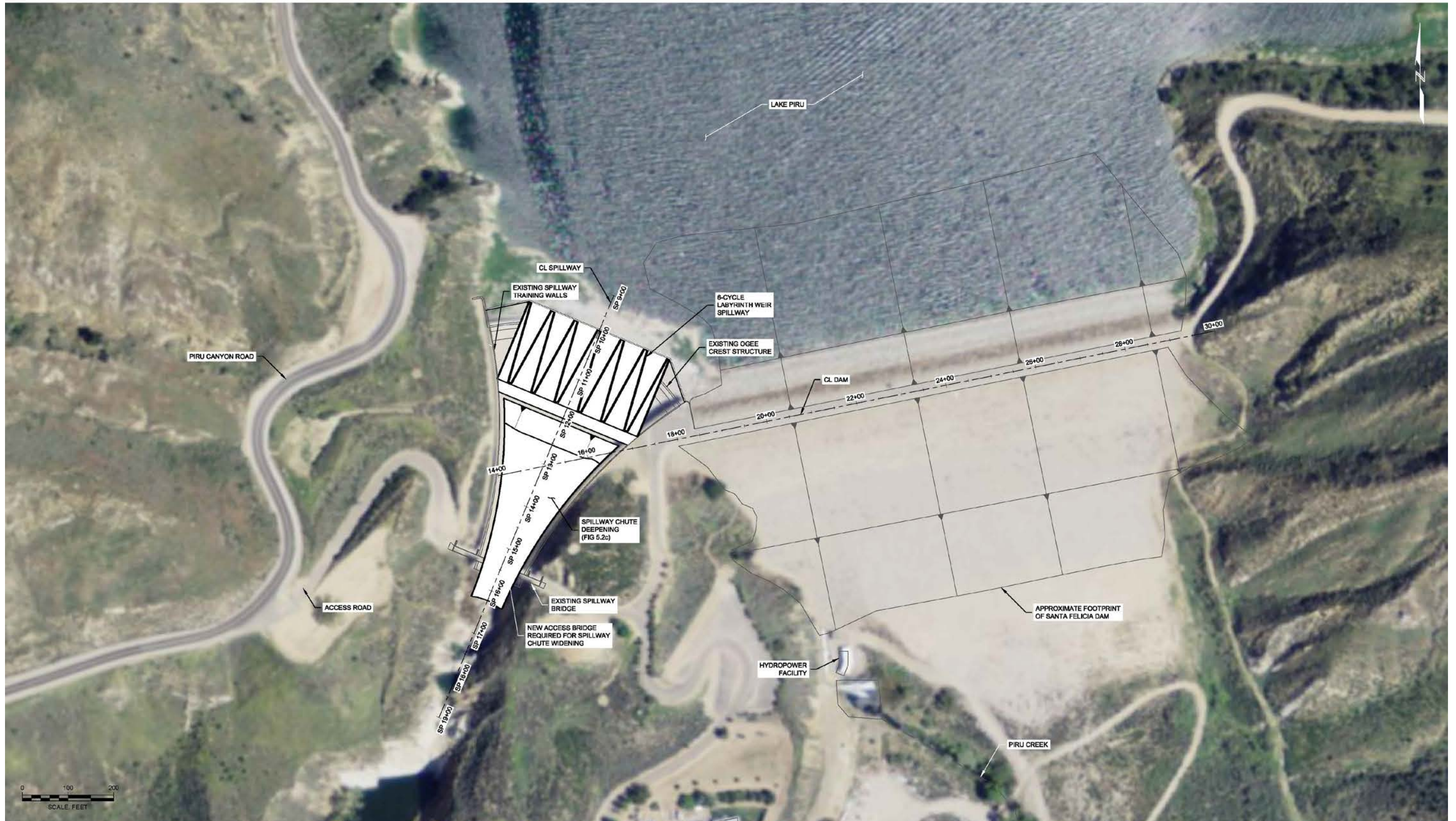
Figure 4-2 Labyrinth Weir Spillway and Spillway Deepening Option
