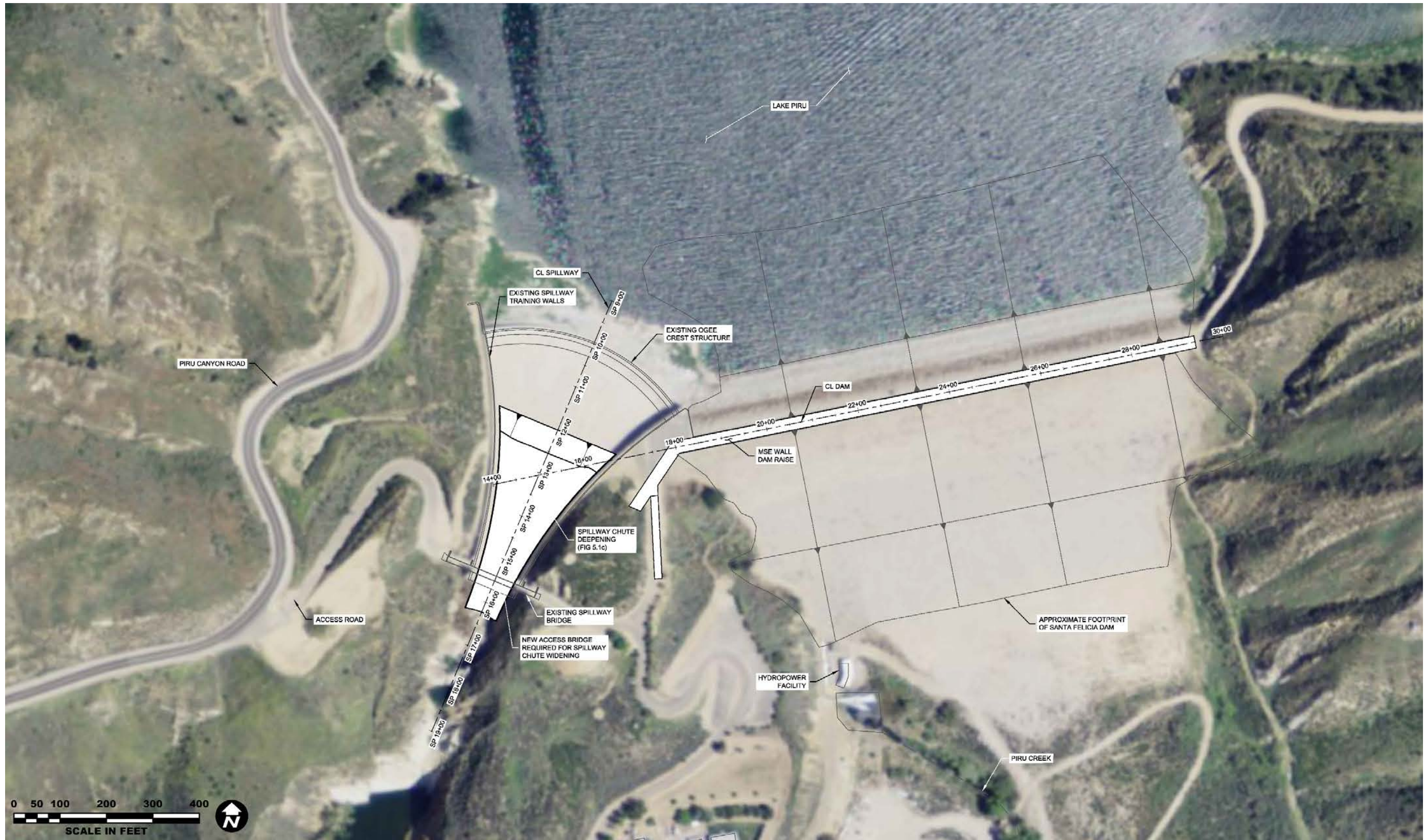
Figure 3-16 Spillway Channel Deepening Option
