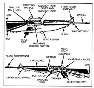
Figure 9-6. Parts of a Rifle
