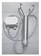
Wind Sensor Wind speed and direction measurements input to aerodynamic model
