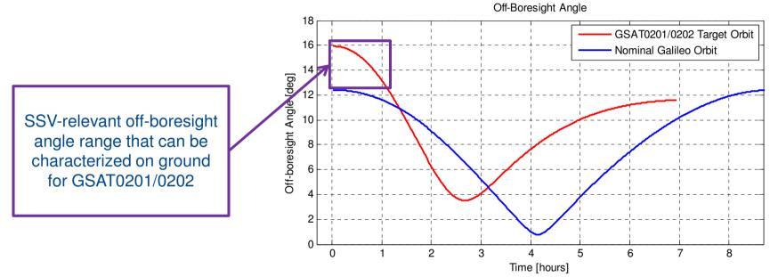
★ Galileo SSV Characterisation up to off-boresight angle of 16° is supported by onground measurements!
