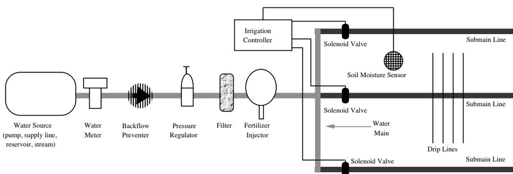
Figure 4.1. Schematic of a recommended drip fertigation system layout for Guam and Micronesia.
