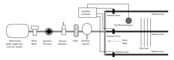
Figure 4.1. Schematic of a recommended drip fertigation system layout for Guam and Micronesia.
