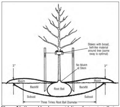
Figure 26. General hardware guidelines for tree installation.
