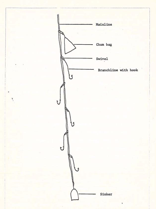
Fig. 16. Diagram of handline showing mainline, chum bag, branchline with hook, and sinker.
