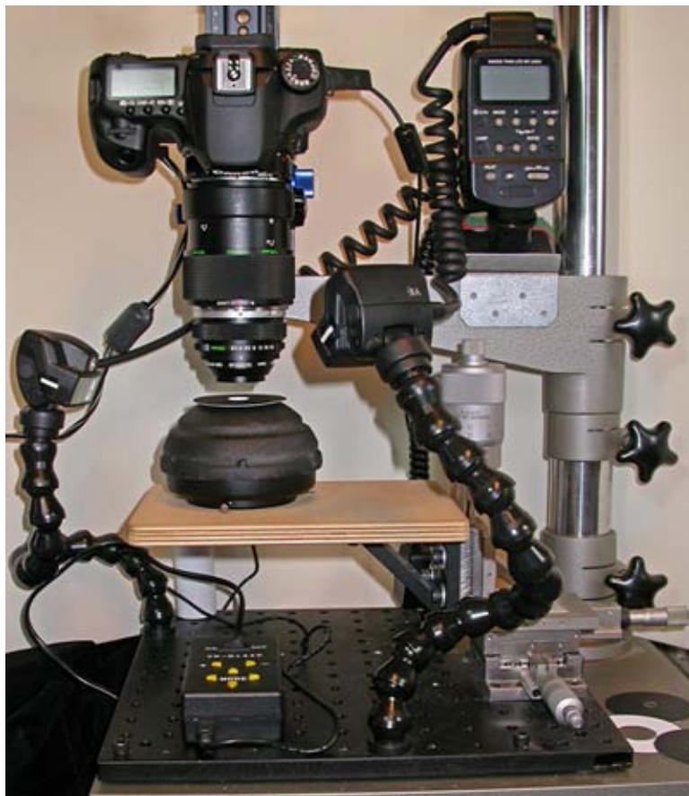
Fig. 5: Photo stand with dome light
