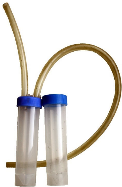
Figure 1 (left). Aspirator with replaceable container - centrifuge tubes. Figure 2 (right). Removing crane flies from the net in the field. Dagestan reserve, Kizlyarskiy region, 24.05.2017. Collection of Erioptera ( Mesocyphona ) bivittata (Loew, 1873) and Idiocera ( Idiocera ) pulchripennis (Loew, 1856) in a sedge-reed-tussock community near an artesian water source.
