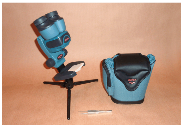
Figure 5. Compact 20x Nikon Naturescope mounted on a Manfrotto Tabletop Tripod. Padded carrying case shown to right and forceps included for scale.
