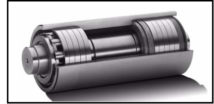
Typical caster foot roll (Uses 2 BR Series Bearings) and re-lube via shaft center
