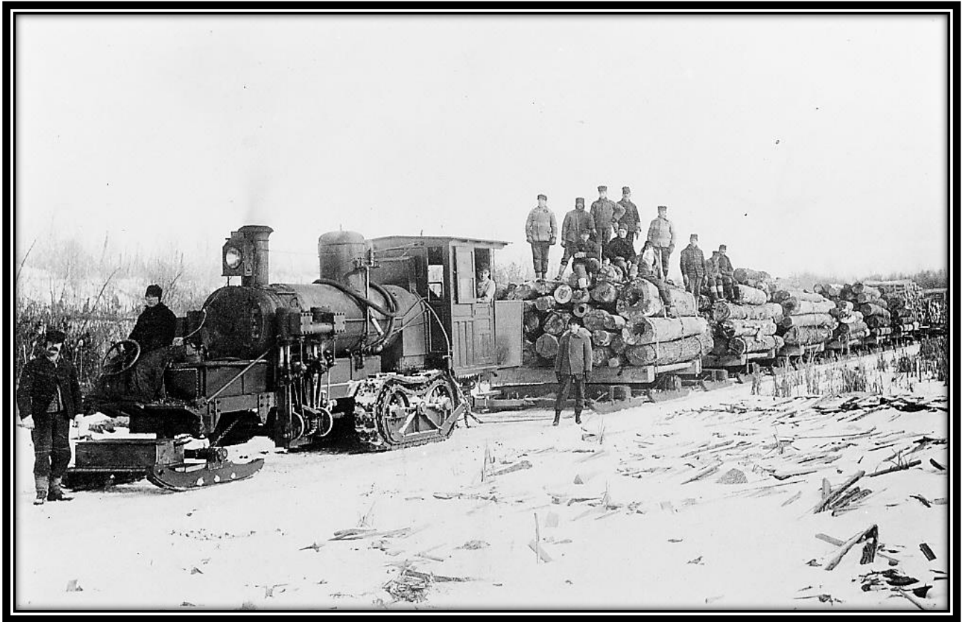
Morgan Lumber & Cedar Company Steam Hauler, Near Foster City, Dickinson County, Michigan, December, 1908: In December, 1908, Foster City's Morgan Lumber & Cedar Company began operating a steam hauling locomotive which could haul from eight to ten loads of hardwood logs each of which would require four teams of horses to pull. Patrick Milligan I stands at the extreme left. At the wheel is "Chicken" Wilson, while Homer Grondine is seated in the cab. R.W. Pierce, company superintendent, stands on the ground in front of the first load. [Beatrice Blomquist]
