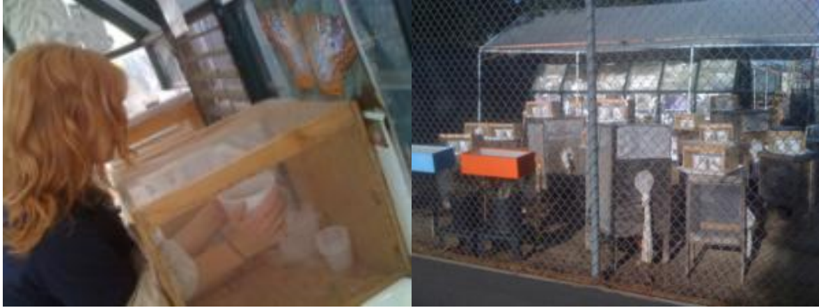
Figure 7. Examples of dual containment. Left: Handling box used for feedings inside greenhouse. Right: Containers inside handling boxes outside in dappled sunlight to stimulate oviposition.
