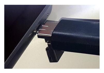
Figure-19: The USB port of the display (option) is situated on the lower edge of the device. Mind the correct position of the connection
