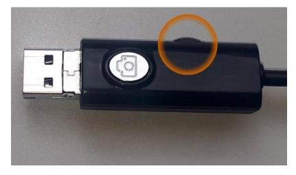
Figure-20: The power of LED lights can be adjusted with the knob (framed)
