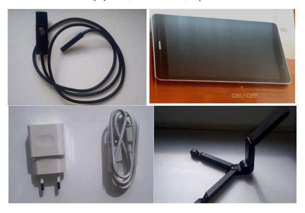
Figure-3: The options of UroStill®. From left to right, from top to bottom: camera, tablet (arrow shows the ON/OFF switch), charger and its cable, stand (unfolded).
