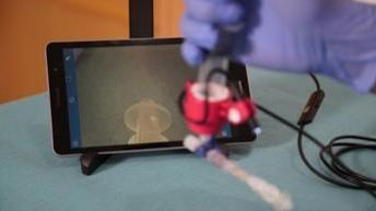
Figure-21 The camera and UroDapter® should be in a parallel position. In this case, UroDapter® appears in the middle of the screen on the display. (To the left: external view, to the right: the image on the display)
