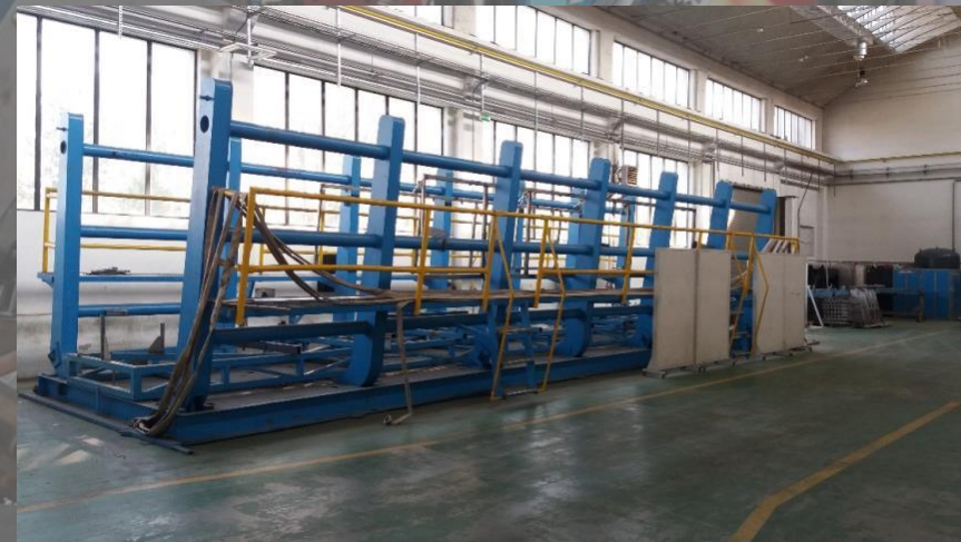
Complete frames welding in main device „Heling”
