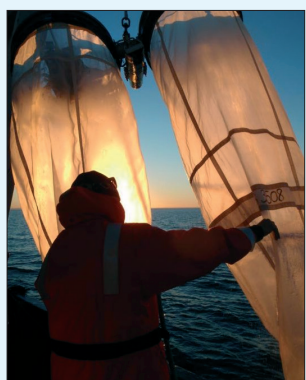
Crew of the NOAA ship Belle M. Shimada recovers the Bongo Net during a CalCOFI cruise.
