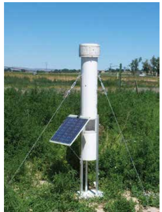
Figure 76. Suction trap for hop aphid. (T.M. Mowry)
