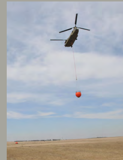
Aircrews from the 11th Expeditionary Combat Aviation Brigade (ECAB) flew three CH-47 Chinooks helicopters, specially outfitted with Bambi Bucket equipment, to assist in the relief efforts of those who were affected by the wildfires, Mar. 9. (Photo by Capt. Matthew Roman)
