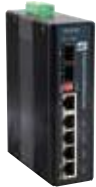
IES-0600 6-Port Gigabit Industrial Switch, 1 x SFP, 1 x SFP/RJ45 Combo, -40°C to 75°C
