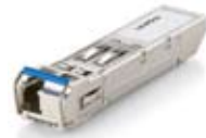
SFP-4330 1.25Gbps Single-mode BIDI Industrial SFP Transceiver, 20km, TX 1310nm / RX 1550nm, -40°C to 85°C
