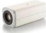
FCS-1160 Fixed Network camera, 5-Megapixel, 802.3af PoE, 12x Optical Zoom, two- way audio
