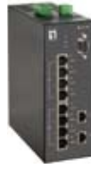
IES-1084 10-Port L2 Managed Fast Ethernet PoE Industrial Switch, 802.3at PoE+, 2 x Gigabit RJ45, 8 PoE Outputs, 181.6W, -40°C to 85°C
