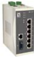
IES-0812 8-Port Fast Ethernet PoE Industrial Switch, 802.3af PoE, 4 PoE Outputs, 1 x SC Multi-Mode Fiber, 61.6W, -20°C to 70°C
