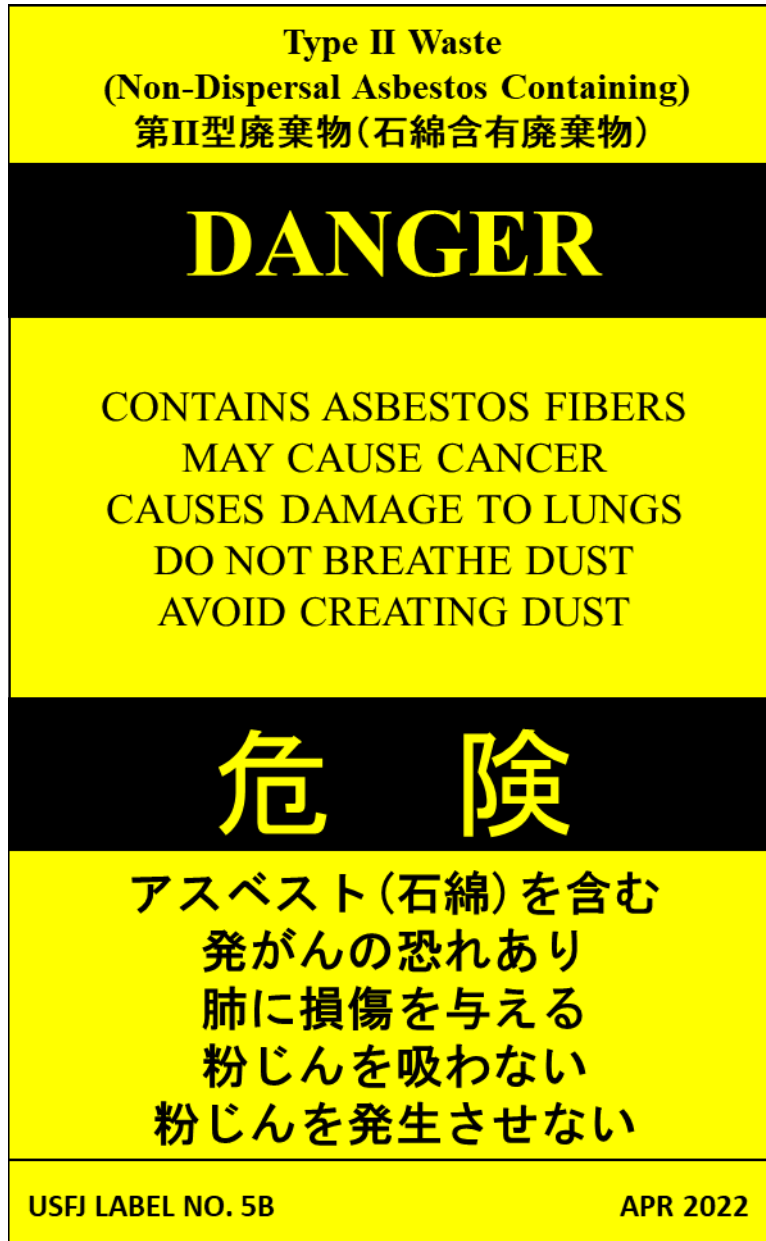
Figure 5.3: Type II ACM Waste Label
