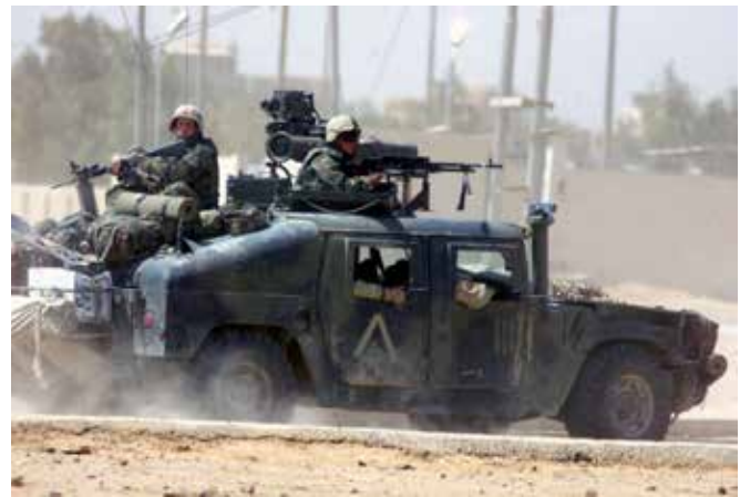
Photo by LCpl Gordon A. Rouse Marines in Nasiriyah mounted on a High Mobility Multi-Wheeled Vehicle (Humvee) designed for the M220 TOW missile launcher and also mounted with a Fabrique Nationale M240G 7.62mm machine gun.
