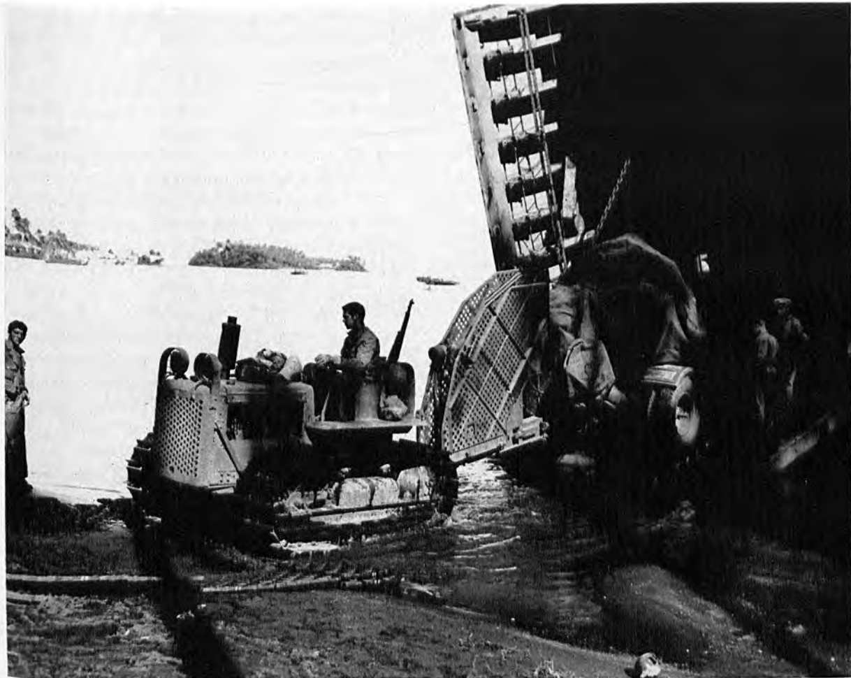
A 90MM GUN of the 9th Defense Battalion rolls down the ramp of an LST beached on Rendova. The TD-9 towing this weapon could not negotiate the mud inland and was in turn towed by a TD-18 nearly twice its size.
